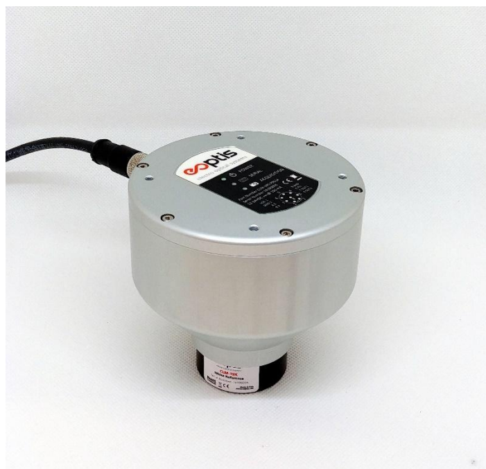
Figure 5: white reference standard positioning for user calibration
